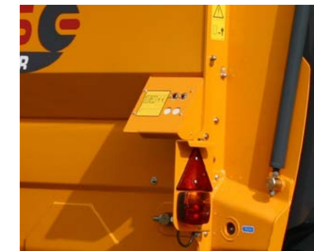
2 nd control unit Control of rear collection door to save time when loading.
